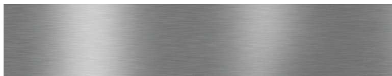
Stainless steel AISI 304 with satin finish.
